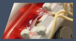
Continuously monitor and control the state of your culture through the integrated sensors for pH, oxygen and biomass
