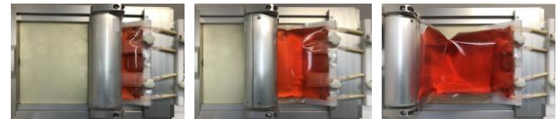
Figure 2 Expansion of the volume of the bag. Minimal volume (left), half the volume (middle) and maximum volume (right).
