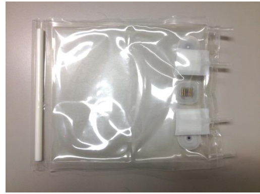
Figure 1 The single-use bioreactor bag of the Scinus Cell Expansion System, with incorporated sensors to the right
