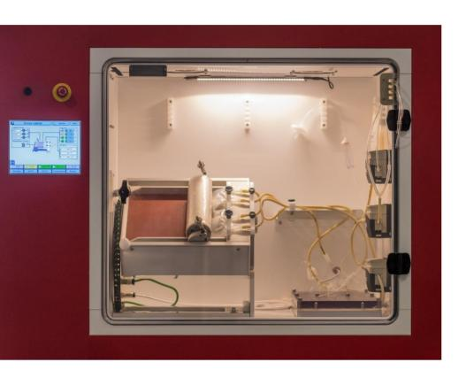
Figure 1 The SCINUS, a bioreactor for large-fold adherent cell expansion
